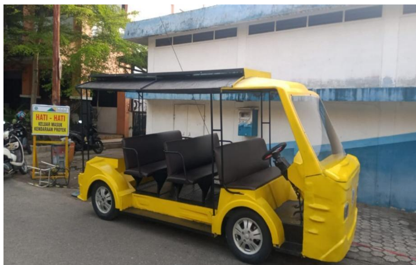
Gambar 4. Prototipe bodi shuttle bus listrik UNP hasil rancang bangun
