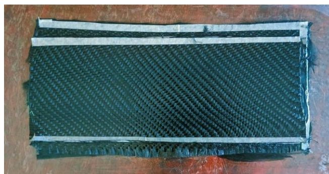
Gambar 5. Proses Manual Hand Lay-Up
